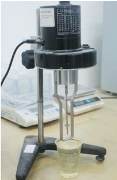
Resin saturation being tested before approval for usage
