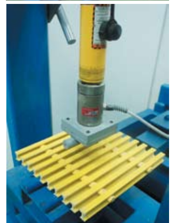
Load / Deflection test conducted at Hexagon Composite own QC premises.
